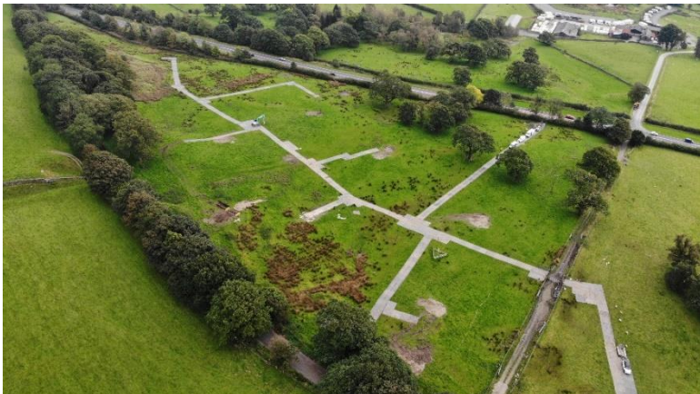
Aerial view of the temporary track way to protect the field.
