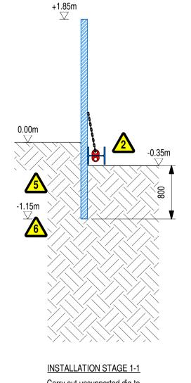
Carry out unsupported dig to -0.35m and place frame into the excavation. Using frame as a guide, place sheets and push to include a
