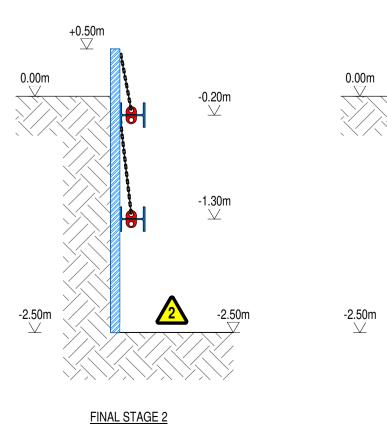
Pump out (F2) at -1.30m and lock off hydraulics. Push sheets to -2.50m and dig to formation level at
