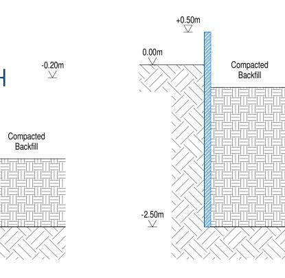
REMOVAL STAGE 3-2 Backfill to underside of (F1) and remove (F1).
