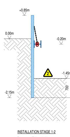
Pump out (F1) at -0.20m and lock off hydraulics.
